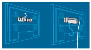
Unit shown mounted directly onto back of flat panel display.
