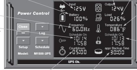
7. Approximate Backup Time: Indicates the approximate amount of backup time that is available, based upon the battery capacity and the load on the system. This indicator can appear in red, any open applications, and then shut down the operating system in an intelyellow, or green, depending upon the number of minutes available.
