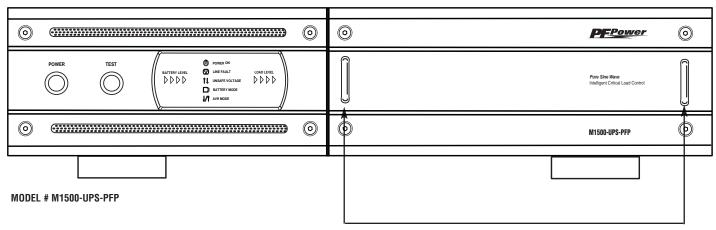
**CAUTION!** The 2 silver handles on the battery access panel are for removing the panel only. **THEY ARE NOT FOR LIFTING PRODUCT.**
