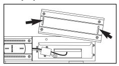
**1.** Remove the right side front panel using pull-out handles.
