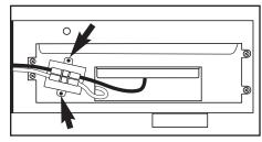
**2.** Remove the two retaining screws of the cable protection cover then remove the cover.
